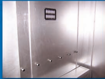
Interior Thermocouple Jack Panel & Vacuum Stubs
